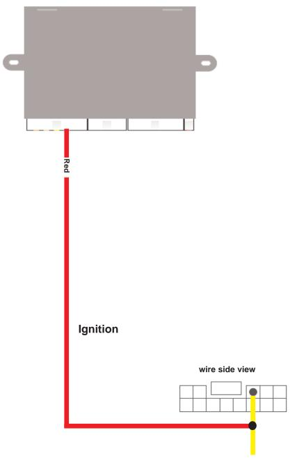
**Connect to Yellow wire at White** connector to the right of fuse box
