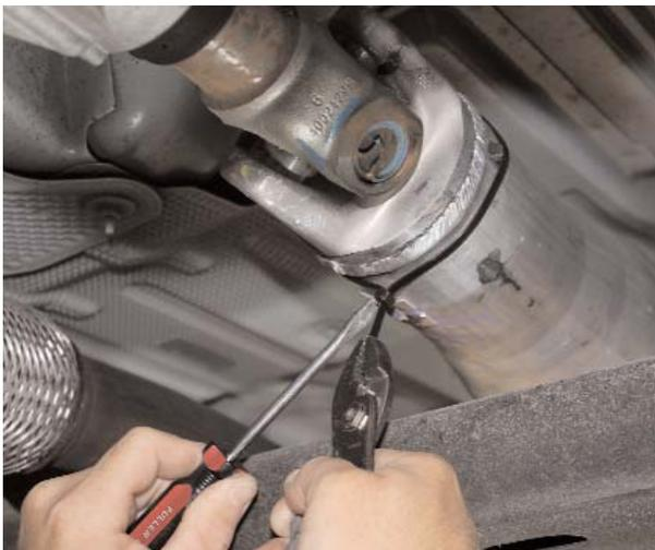
3. Using flat head screw driver and pliers crip down tie strap to secure magnets
