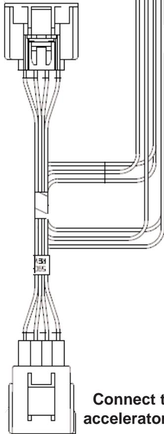
Cut off ground terminal on Black wire of cruise harness. Then solder and tape Black wire to position 1 of the accelerator pedal interface connector Black/White wire for ground as shown in picture below
