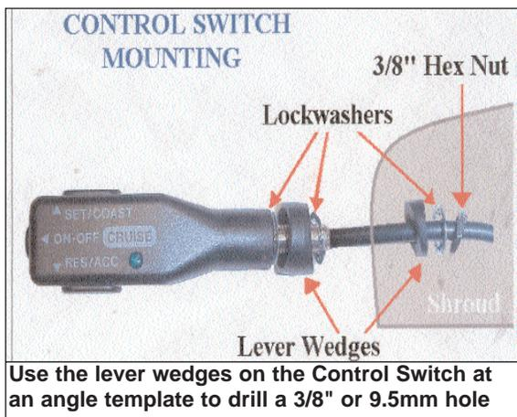
Use the lever wedges on the Control Switch at an angle template to drill a 3/8" or 9.5mm hole
