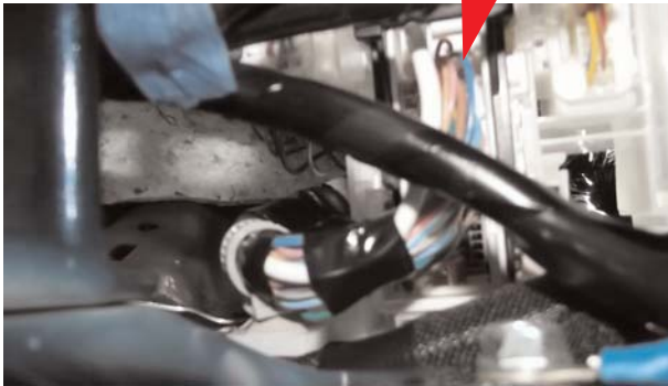
Above drivers kick panel locate 18 pin white connector in position 17 connect red ignition wire to LT Green wire from ignition
