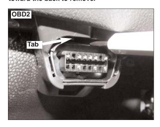
Connect Red wire to White/Blue wire in Pin 6 and Connect Black wire to White wire in Pin 14
