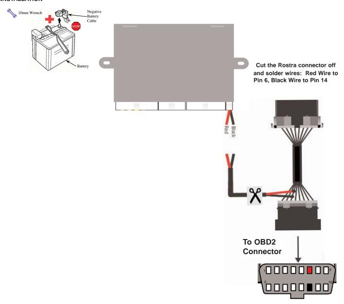
Note:Use a precision tool to press up on the backside of the OBD2 connector housing to release the tab. Push out OBD2 connector toward the back to remove.
