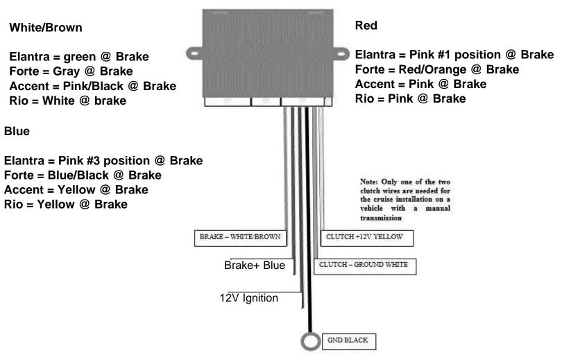
Note: Both brake wires must be connected for cruise to operate. White/Brown must see ground at rest and battery voltage when brake is applied. Blue must see constant battery voltage from brake system.
