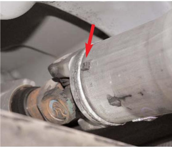
1. Mount 2 magnets on the driveshaft 180 degrees apart using epoxy in cruise package.
