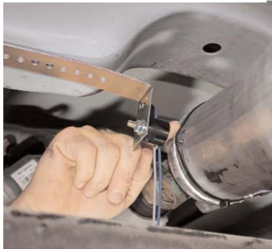
4. Position the pickup coil face between 1/2" to 1" away from the magnets on drive shaft staying directly inline with magnets
