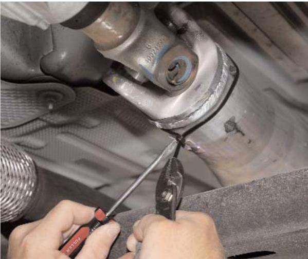
3. Using flat head screw driver and pliers crip down tie strap to secure magnets
