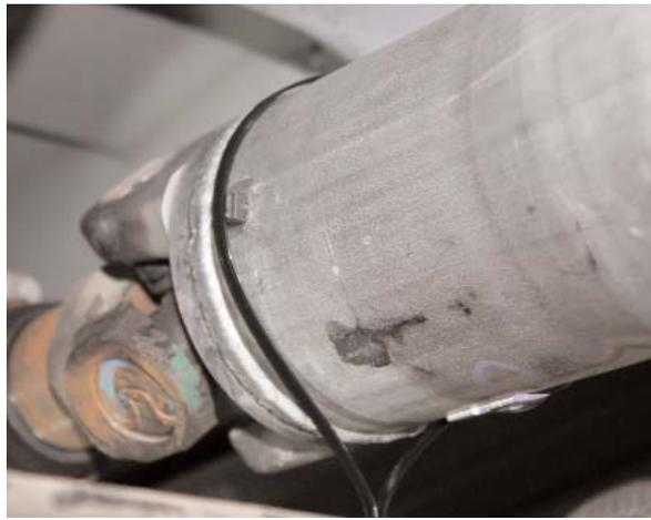
2. Place tie strap around drive shaft over magnets from cruise pack
