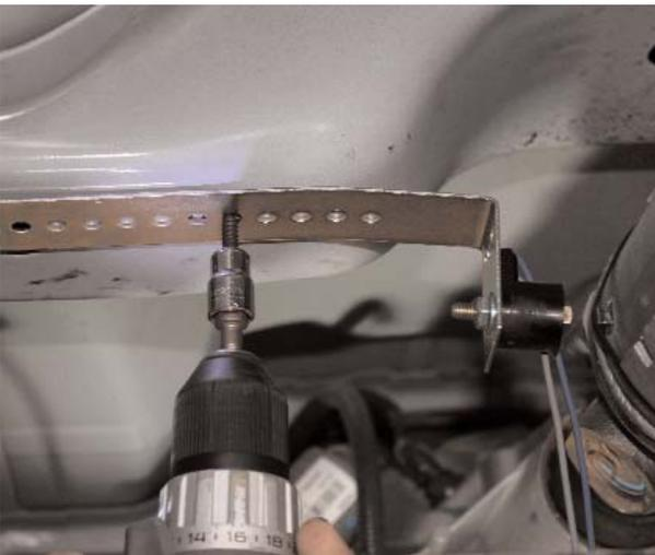
5. secure magnet coil bracket with supplied self tapping screws in kit.
