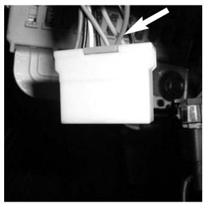
Hyundai Accent: Connect the Red Ignition wire to pink wire in top left corner of white connect on the left side of the fuse box located under the drivers side dash
