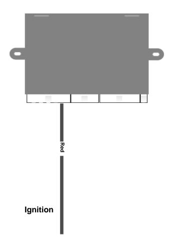
Kia Rio: Connect the Red Ignition wire to orange wire (between gray and yellow wire) as shown at the traction control connector located behind the drivers side dash.
