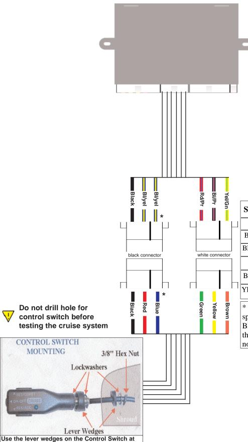
an angle template to drill a 3/8" or 9.5mm hole
