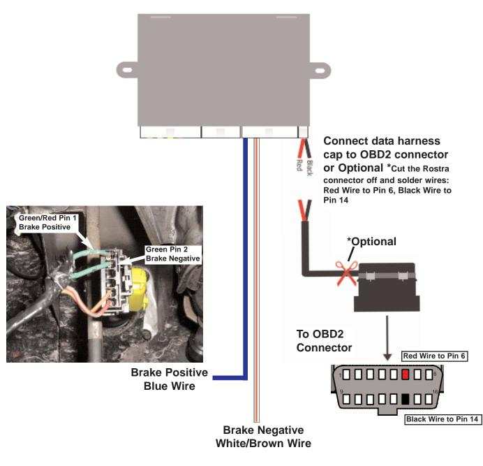
Note: Only use the wires listed in the instructions for Main Wiring Harness connections. All other wires are not used.
