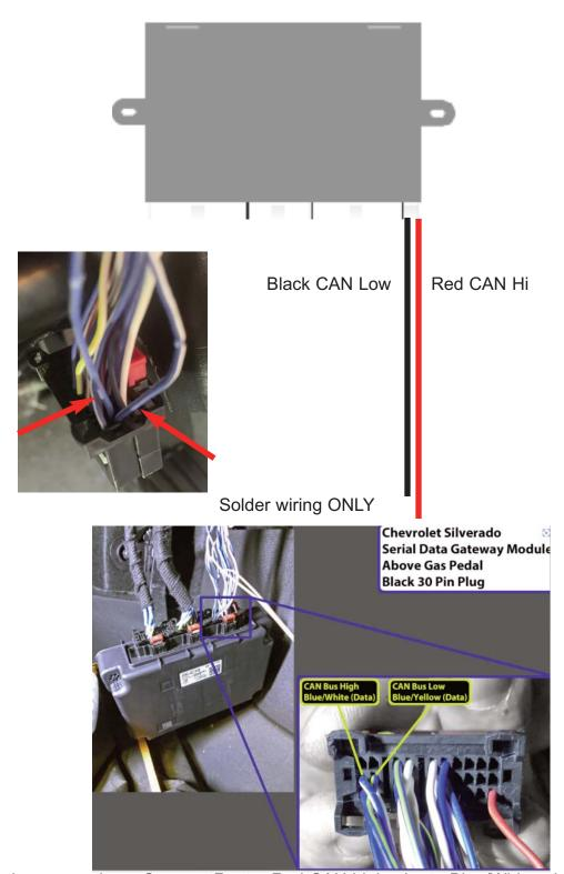
CAN wire connections: Connect Rostra Red CAN high wire to Blue/White wire in position 20 of Serial Data Gateway above accelerator pedal. Connect Rostra Black CAN low wire to Blue/Yellow wire in position 19 of Serial Data Gateway above accelerator pedal.
