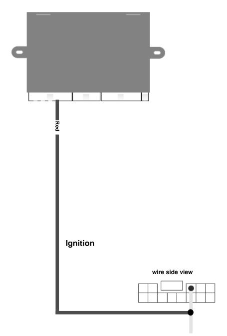
Connect to yellow wire at white connector to the right of fuse box
