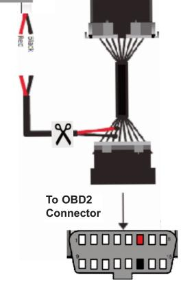
Note: Standard OBD2 Connect Red wire to White/Blue wire in Pin 6 and Connect Black wire to White wire in Pin 14
