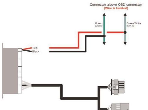
Connector on the accelerator pedal
